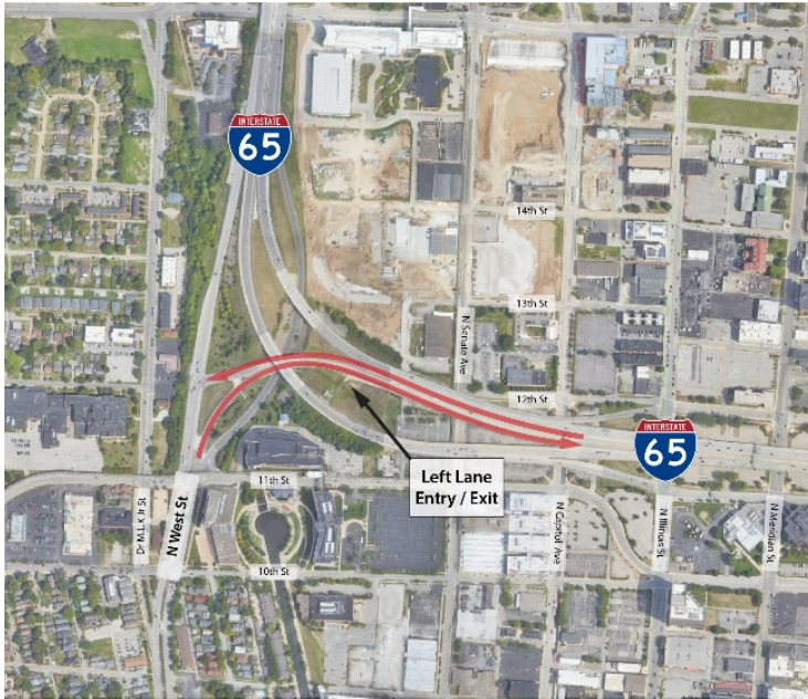
Figure 5: Geometric Deficiencies at I-65/West St.
